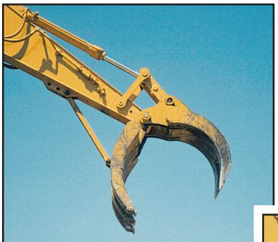
Empire Bucket's Grapples are built to handle the ever increasing demands of demolition and recycling - heavy duty designs give you a high amount of tooth overlap to compress your load, leaving behind dirt and small rocks.
