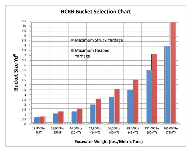
Contact your dealer or Empire Bucket to determine the maximum capacity for your excavator (must consider excavator size, bucket weight and capacity, material weight, other optional equipment on your machine such as couplers, thumbs, etc.) Larger capacity buckets may be possible when working in light materials, for flat or level applications or mass excavation applications where material being loaded only. Smaller capacity buckets are recommended for more adverse working conditions.
